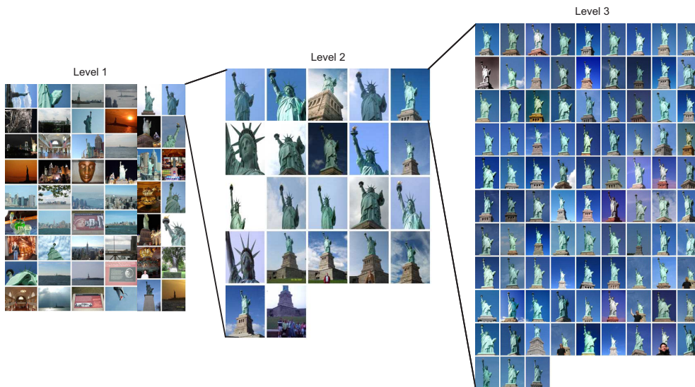
Fig. 21 Hierarchical organization of the dataset for browsing. Level 1: components of the iconic scene graph. Level 2: Each component can be expanded to show all the iconic images associated with it. Level 3: each iconic can be expanded to show the images associated with its gist cluster. Our three datasets may be browsed online at www.cs.unc.edu/PhotoCollectionReconstruction .
