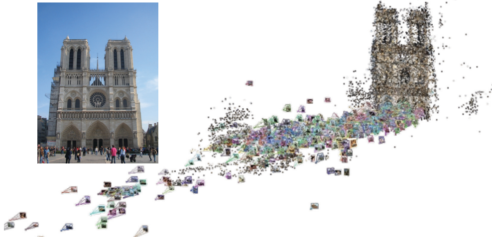
(a) The front side of the Notre Dame Cathedral (1300 cameras, 65022 3D points, 1121931 2D projections).
