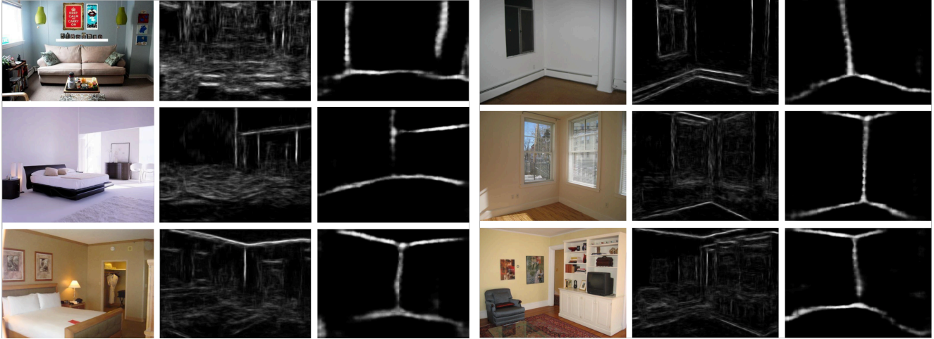
Figure 3. Comparison of Informative Edge Maps generated by the Structured Forest and the FCN. Each triplet of images from left to right, top to bottom shows the input indoor scene, the output of the 1 Class Forest trained on the SUNbox dataset ( Forest-1 Class-SUNbox ), and the 1 Class FCN trained on the Hedau+ dataset ( FCN-1 Class-Hedau+(Joint) ). Note that the FCN produces good edge maps even in the presence of clutter such as the couch and the bed in the images above.
