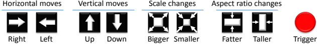
Figure 2. Illustration of the actions in the proposed MDP, giving 4 degrees of freedom to the agent for transforming boxes.
